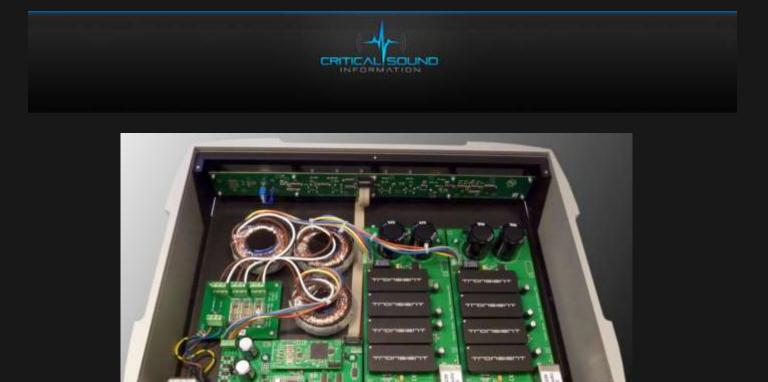
There are no shortage of parts inside Pavane, either in number or quality. While most engineers would have used a DAC circuit to convert the signal, sitting here are eight ! First, Pavane is built with dual mono construction, with separate power supplies and circuit boards to each channel. A third power supply takes care of the other logic circuits.
