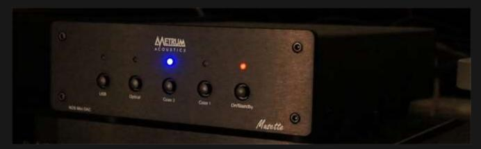
As with most other DAC's there are USB, Optical Toslink and then two Coaxial / SPIF inputs. USB drives up to 384 kHz sampling, SPDIF up to 192 kHz and Optical up to 96 kHz. Analog output supplies the normal 2 volts with a very low distortion of 0.007% THD.
