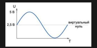
Firstly, the classical R2R scheme disadvantage is the problem of so-called "virtual zero" (conversion of a variable sound signal), which appears at the moment where the transformation matrix AC audio signal is an average value of output voltage equal to half the supply voltage. These points in the circuit must be switched all at once and even a slight asynchrony in their shift for example (because of the magnitude of the deviations of resistances), leads to disruption of the conversion process.
