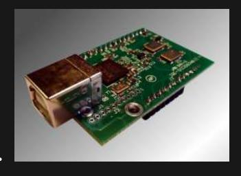
The quality USB-module uses a modified production *M2Tech* unit, similar to that installed in the latest model of the famous Italian firm hiFace Evo Two. The module operates in an asynchronous mode, equipped with a pair of high-precision clocks and supports digital signals with a frequency up to 384 kHz. As I mentioned, this module is USB powered from a separate internal power supply in order to prevent ingress of noise and interference through the USB-powered interface.
