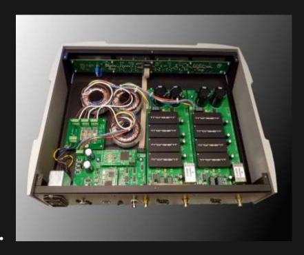
Much attention was paid to the power supply system, for high quality power is required - a prerequisite for accurate digital to analog conversion. At the input a Schurter power line filter is installed. The design uses three separate toroidal transformers for better power ; one for each channel and the third - for the USB module and control circuits. The power supply circuit for each channel - a pair of 22,000 uF capacitors.
