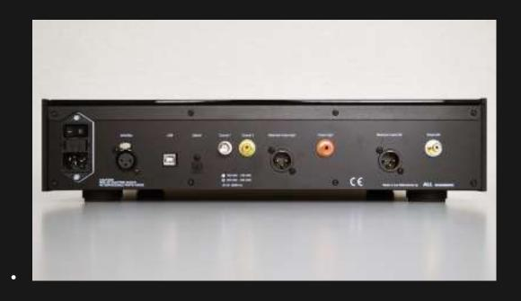
Digital inputs : AES / EBU, Coaxial BNC and RCA - in order to avoid unwanted interference connections are galvanically isolated.
