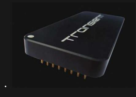
As a result of these two innovations a unique converter module has been developed - *Transient*, having properties previously unobtainable to R2R circuits - high linearity conversion in the weakest of signal information down to -140 dB, low noise and distortion.
