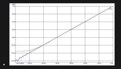
The graph shows that the linearity of the *Transient* module for weak signals (blue and red lines) greatly exceeds the capabilities of modern chips with oversampling (green line).
