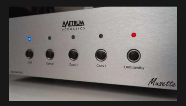
Connectivity options: Optical, Coaxial and USB-B selects the input gear.
